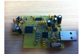
**Figure 3. USB hub, PIC, current sensing and virtual sensor circuitry**
