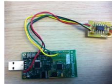
**Figure 2. TelosB mote (left) and optocoupler board (right) which are housed within the PEN.**
