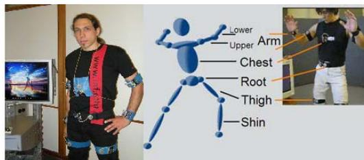
**Fig. 1.** On the left a student wears the 10 sensors and the computer displays his avatar in real time. The right shows the avatar bones model and relationship of sensor to limb.
